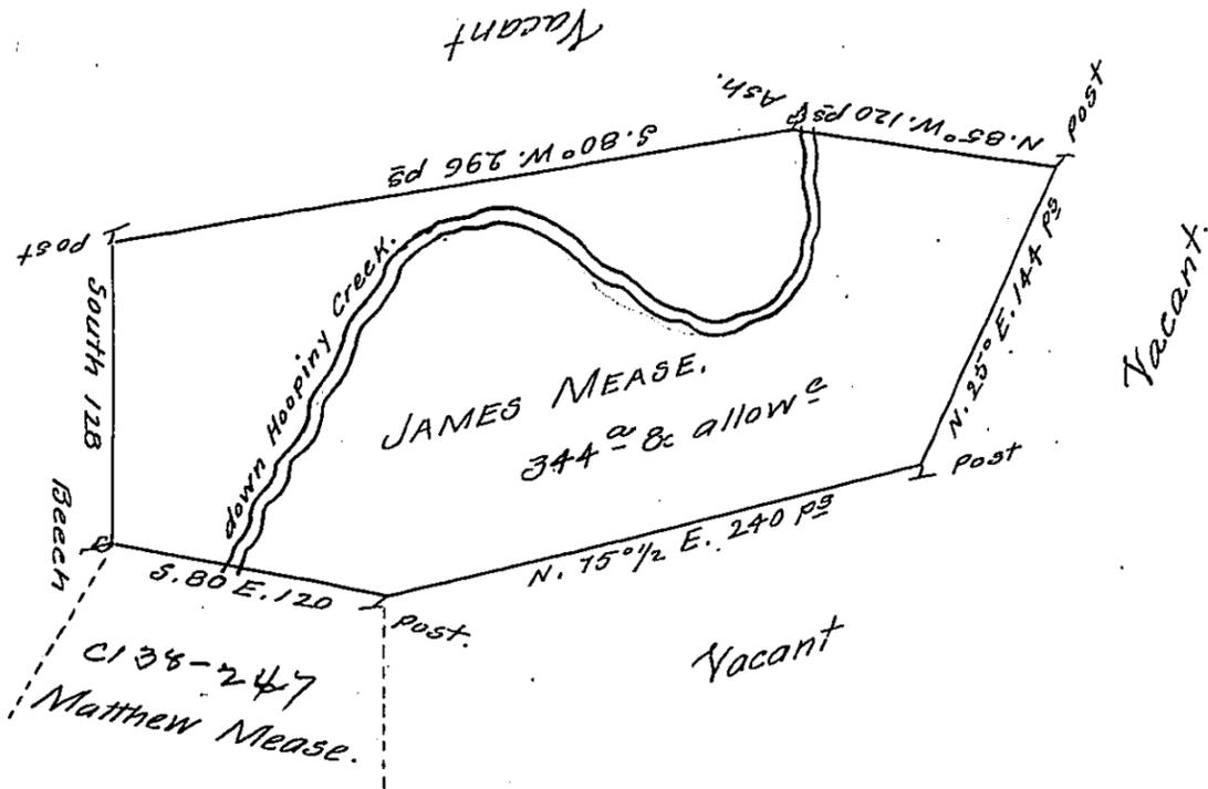
A Draught of a Tract of Land Called — situate on both sides of Hoopiny Creek about four Miles and a half from the mouth including an Ash Tree marked with four Notches & two Blazes Standing on the bank of the Creek in the County of Northumberland Containing three hundred and forty four Acres besides the usual allowance of six Cent for Roads &c. Surveyed the 6th Day of October 1774 For James Mease In pursuance of a Warrant dated the 15th day of June 1774 by
